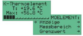
The function menu includes different windows for presenting your measured data. In the overall display, the measured values of all active measurement channels are displayed in parallel rows that can be scrolled up and down in a window. In the individual display, you can configure an individual display window for each
